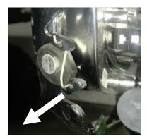
7. For the driver side, it will require removal of the headlight subframe. Gently work the outboard headlight mount until it is almost able to be slid out. Remove two T25 bolts per side of the subframe bracket. As the bracket is being removed, support the headlight and carefully demount the light from the subframe. Now, remove the headlight.
