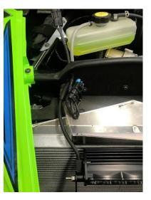
15. If you have purchased the additional Baja Designs Textron Wildcat Headlight kit (44-7094, 44-7095, 44-7096), skip steps 15-16. Now it is time to remount the stock headlights. Beginning with the passenger side, place it into the opening as shown below. Align the headlight mounts and the tilt adjuster assembly simultaneously. It may be necessary to bend the U-bracket slightly for the next step.
