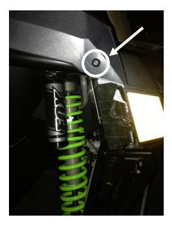
4. Now, at the front of the vehicle, locate the two pressed in black plastic fasteners near the front corners of the hood opening that secure the grill. Using a standard screwdriver, pry up the center section until it appears as shown below.
